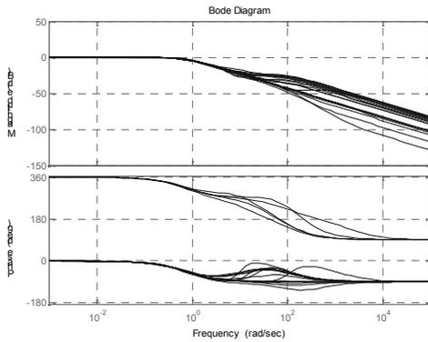
**Fig. 9.** Frequency response of the tail motor.
