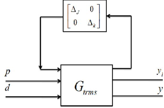
Fig.6. LFT representation of perturbed Two input two output systems
