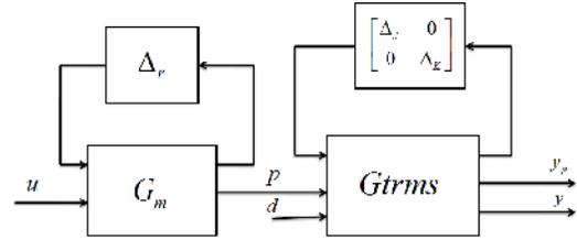
**Fig.11.** Uncertainty modeling of Twin Rotor MIMO system with motors (main and tail motor).
