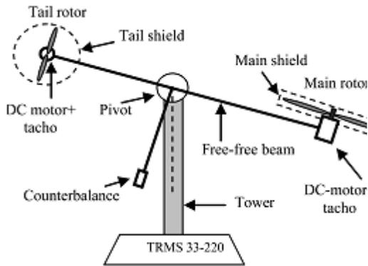
Fig. 3. Twin Rotor MIMO system.
