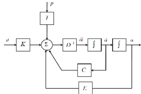
Fig. 4. Block diagram of Twin rotor MIMO system.
